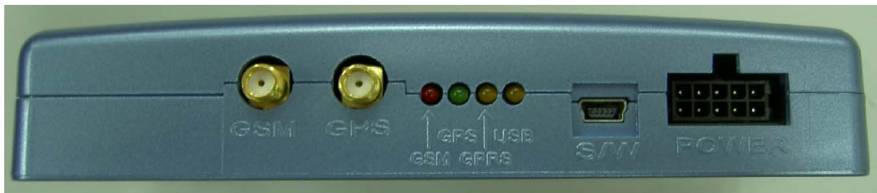
Rear connectors of MightyGPS iTrack Gold
